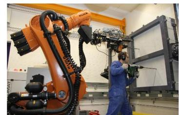
*The Power Tool Test Lab allows for reproducible test conditions in product development. (Photo: IPEK, KIT)*
