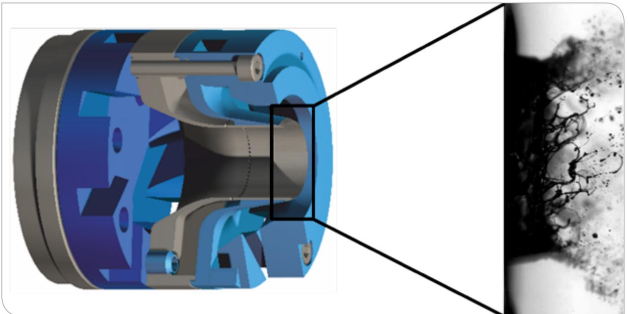
Typical injection nozzle and photography of the atomization process
