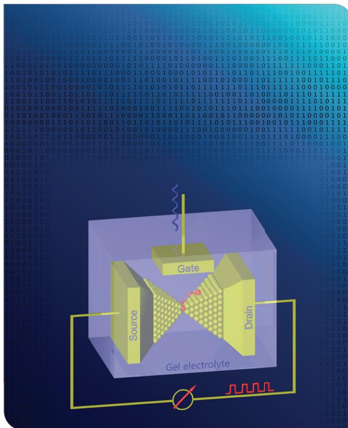
Schematic representation of the mode of operation: In the single-atom transistor, a very low control voltage at the gate electrode moves a single atom in a controlled manner, thereby closing or breaking an electrical circuit (Image: Research Group Professor Thomas Schimmel/KIT).
