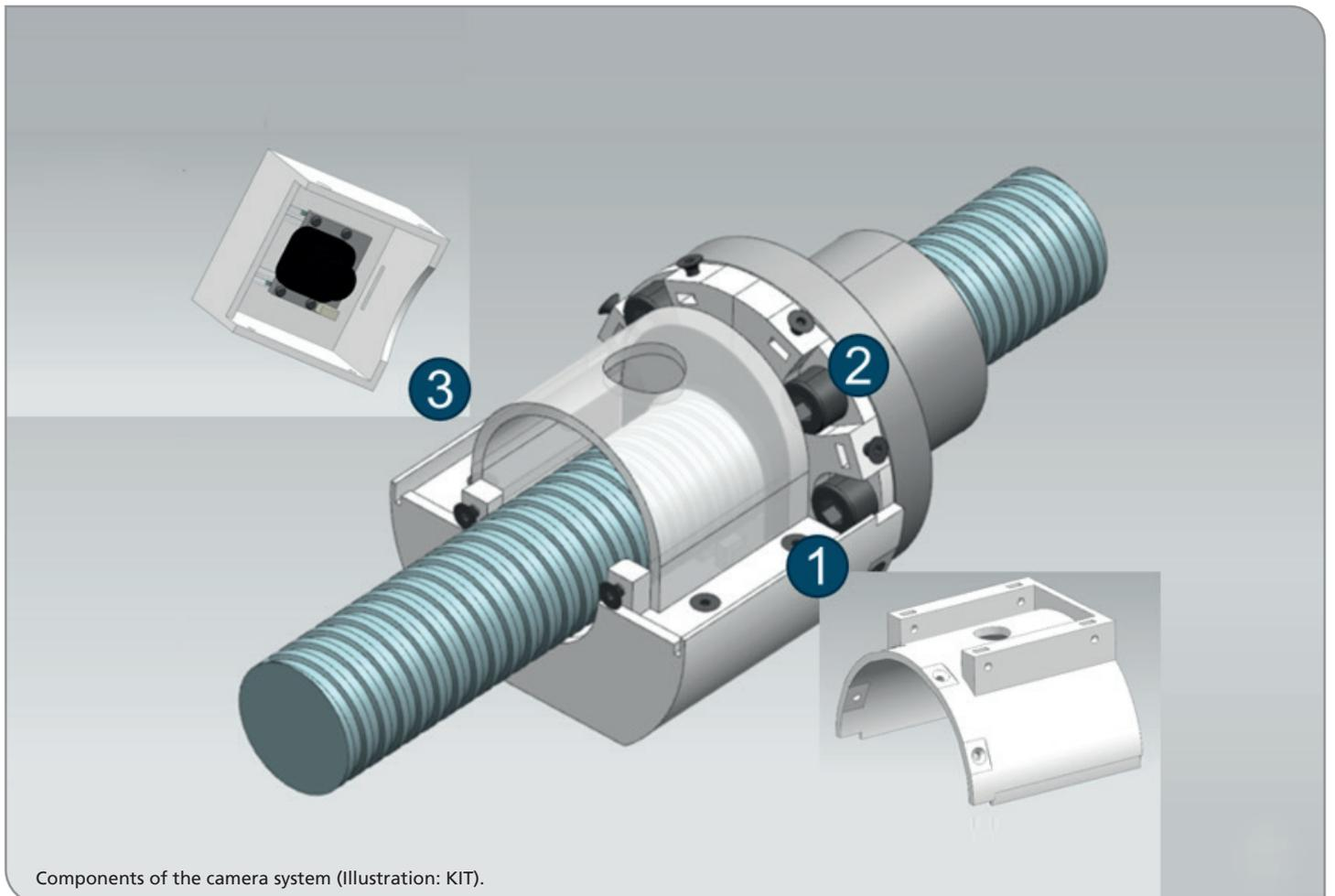
Components of the camera system (Illustration: KIT).
