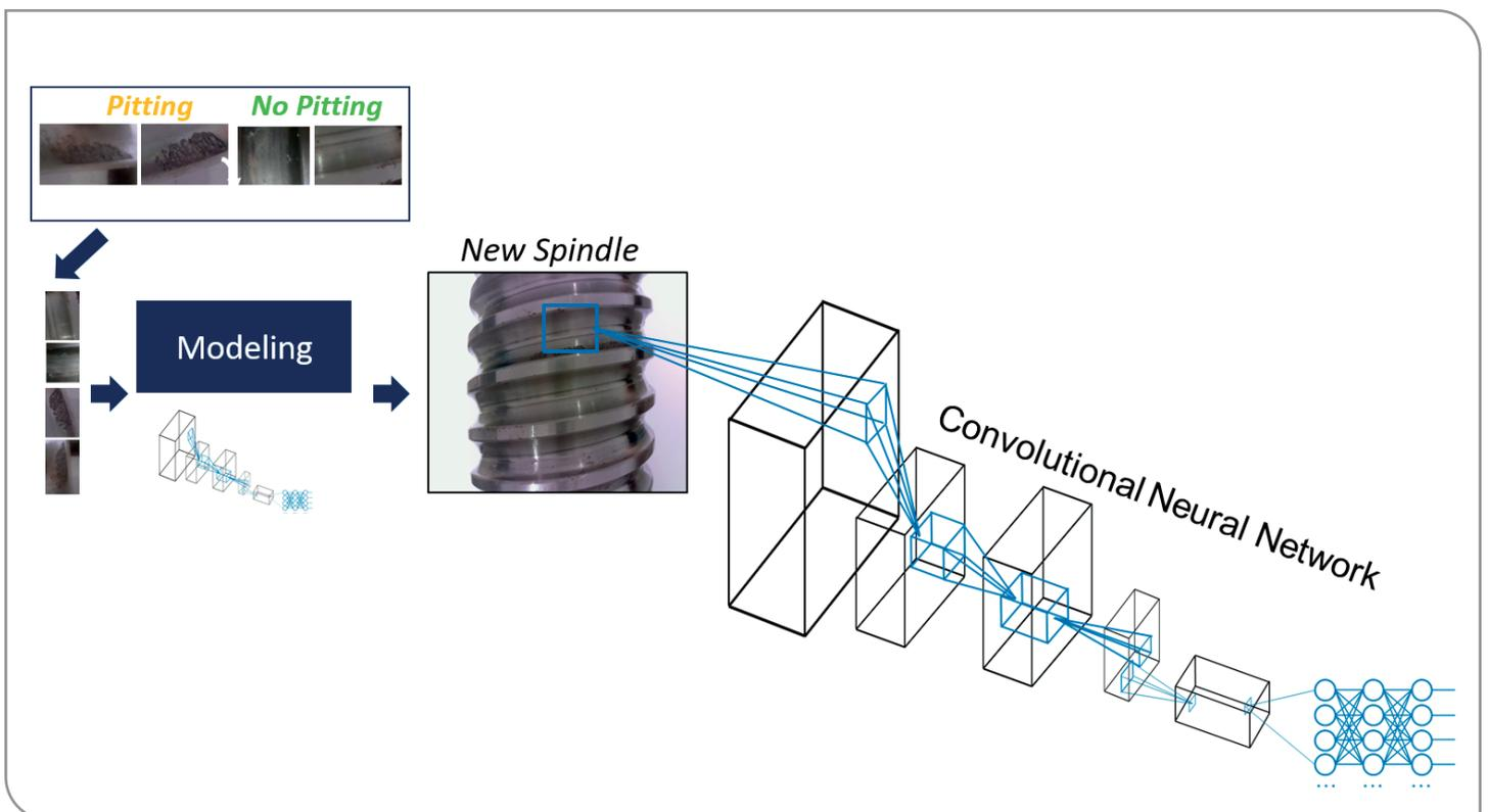
Basic functioning of the smart image evaluation model (Illustration: KIT).
