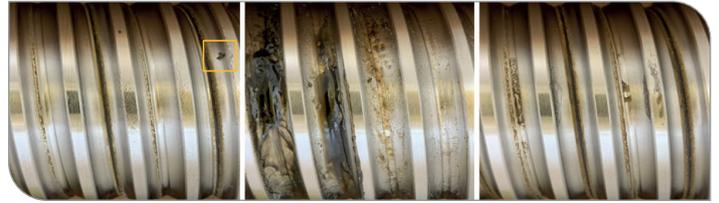
Spindle states: Left: Small pitting, middle: Heavy contamination, right: Pitting-like contamination (Photo: KIT)
