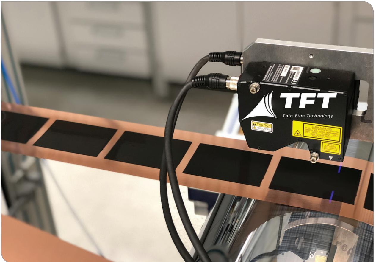
Inline measurement of the electrodes ensures highest quality.
