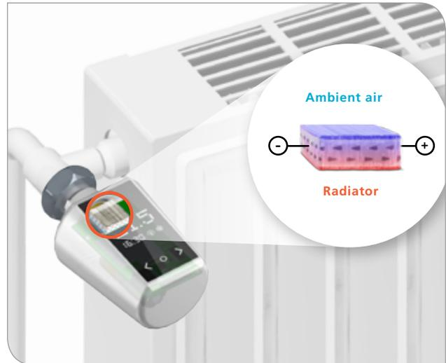
Thermoelectric generators for the autonomous supply of measurement electronics, such as a smart radiator thermostat
