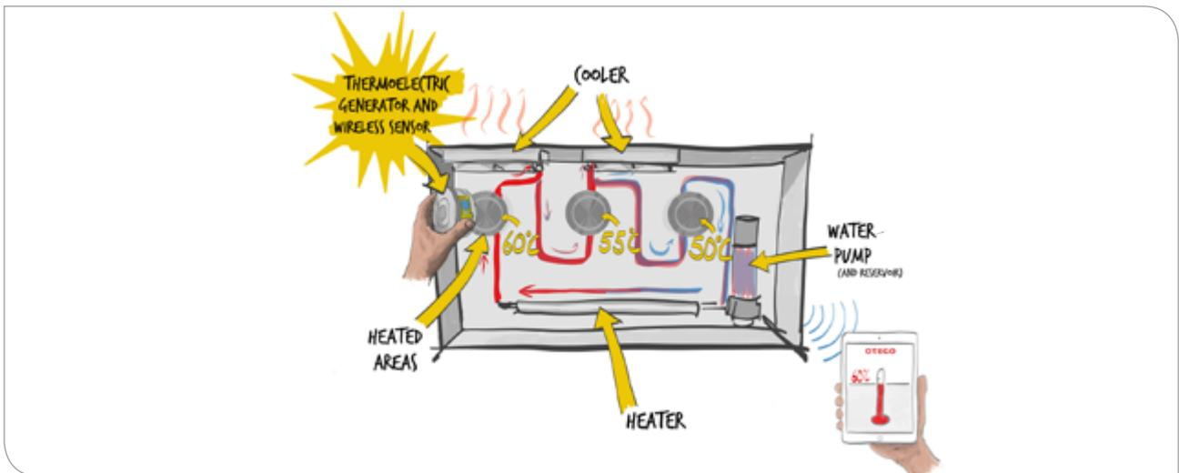
Exhibit at Hannover Messe 2018: A water circuit as heat source supplies sensor pucks with energy. This is enabled by otego's thermoelectric generators that directly convert waste heat into electric power
